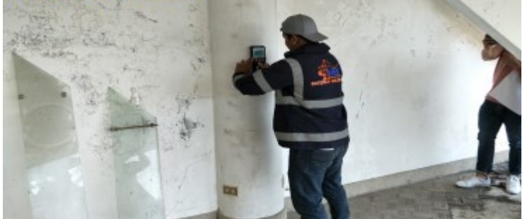
STRUCTURAL ASSESSMENT & INTEGRITY CHECKING OF EXISTING EXISTING MONTERRAZAS CLUBHOUSE AT ITOGON, BAGUIO CITY NON-DESTRUCTIVE TEST REBAR SCANNING
