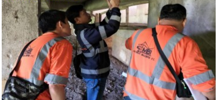
STRUCTURAL ASSESSMENT & INTEGRITY CHECKING OF EXISTING EXISTING MONTERRAZAS CLUBHOUSE AT ITOGON, BAGUIO CITY NON-DESTRUCTIVE TEST REBOUND HAMMER
